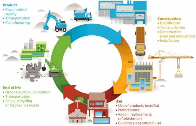
Figure A3-9: The Life Cycle Assessment of a Construction Product
