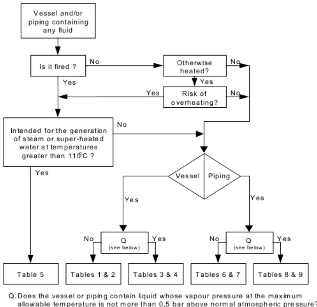
Figure 2.1: Classification of equipment under the PED<sup>9</sup>
